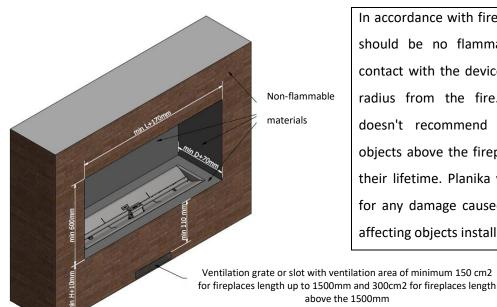
In accordance with fire safety measures there should be no flammable objects in direct contact with the device nor within a 1 metre radius from the fire. Additionally, Planika doesn't recommend placing heat-sensitive objects above the fireplace as it may shorten their lifetime. Planika will not be responsible for any damage caused by high temperature affecting objects installed above the fire.
