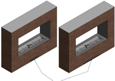
The dimensions and shape of the ventilation grid may be designed according to client specifications however both the minimum ventilation area of (150 cm2 for fireplaces length up to 1500mm and 300cm2 for fireplaces length above the 1500mm) as well as minimum distance from the edge of the housing of 110 minimum need to be observed.
