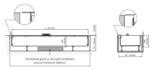
• Prepare the cavity for the insert according to the below scheme. When preparing the cavity take into account that the surface on which the insert is going to be placed needs to be well-levelled as the adjustable supports have a limited range of levelling of the insert. The delivered device is already levelled.
